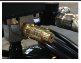
valve discharges air, please turn off the compressor and contact the helpline. The safety valve is located to the side of the pressure switch.
